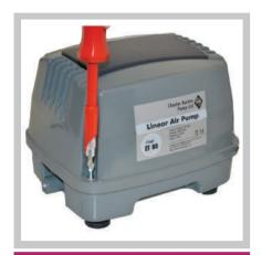
Unscrew the four corner screws and remove the cover from the air pump.
