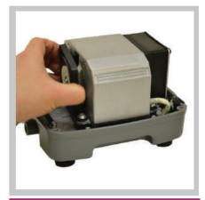
Remove the screw along with the diaphragm depressor, electrostatic membrane and diaphragm. Repeat on the opposite end of the pump
